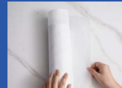
2. Wrap the substrate with a piece of protective paper;
