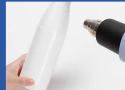
4. Heat the shrink film to make it fit tightly with the substrate;
